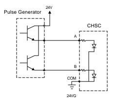
2) Open collector output pulse generator
