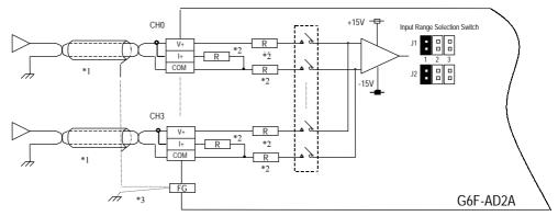
\*1 For the cable, use a two-core twisted shielded wire.
