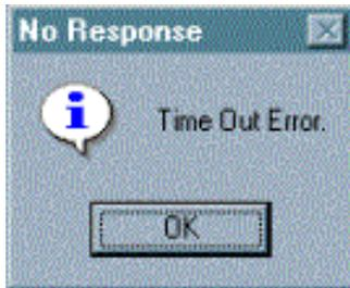
If the message above is displayed, RS-232C cable between PC and PLC may not be connected, or the connection status may be abnormal. Check the connection status of RS-232C cable to verify that RS-232C cable is correctly connected with loader port of PLC CPU.
