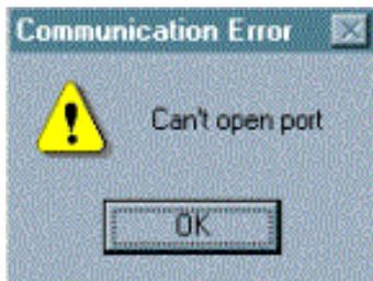
If the message 'Can't open port' is displayed, check communication port setting in option menu of Frame Editor if set as repeated with the mouse or other devices, and then try re-connection.
