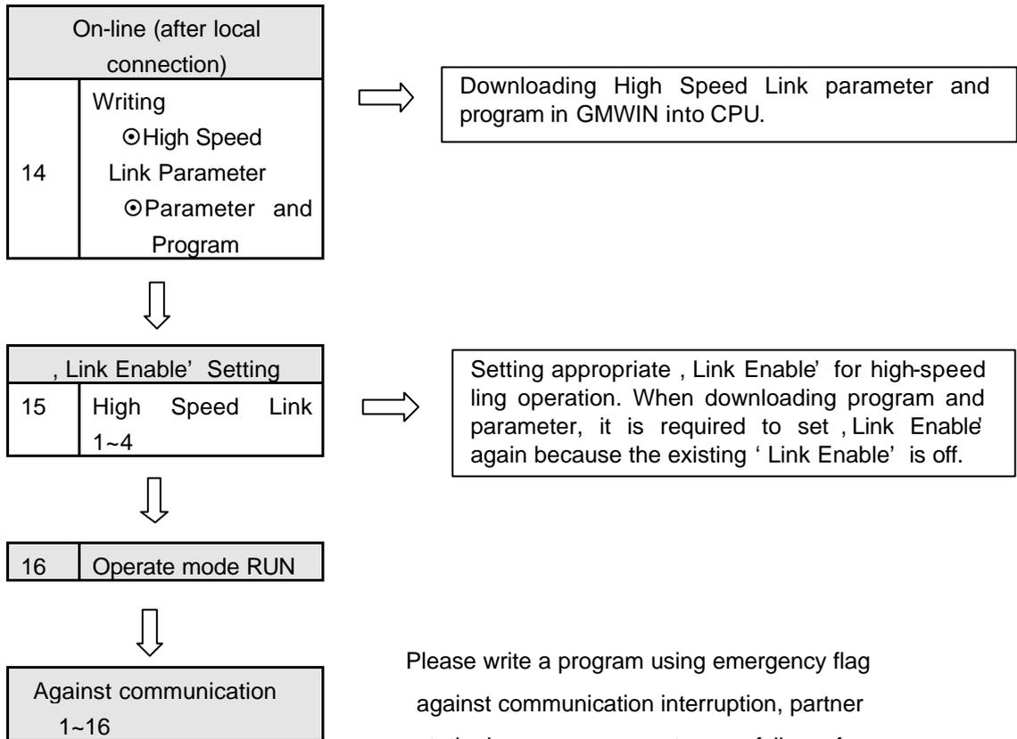
Please write a program using emergency flag against communication interruption, partner station' s error, a moment power failure of remote module at time of communication.
