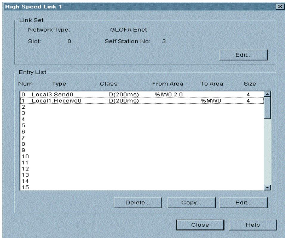
c. Parameter of High Speed Link of GM3 (Station 3)
