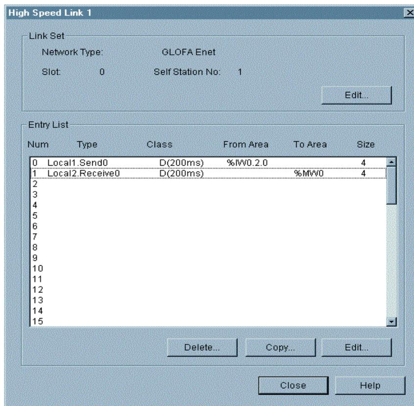
a. Parameter of High Speed Link of GM1 (Station 1)
