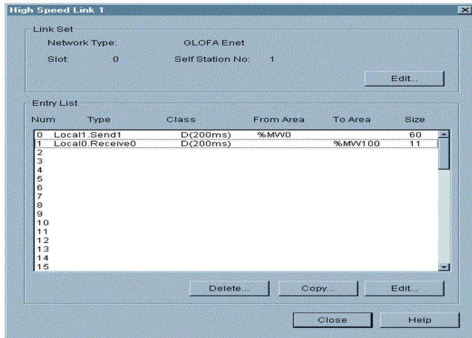
F) Now, select , Close' after setting HS\_LINK parameter setting of the first Enet communication module. For the second communication module, please set HS\_LINK via the process from A to E. At this time, select HS\_LINK 2 and slot number 1, and save saving area of RX data %MW200 not to be doubled with the saving area received in the first module. After setting, following screen appears.
