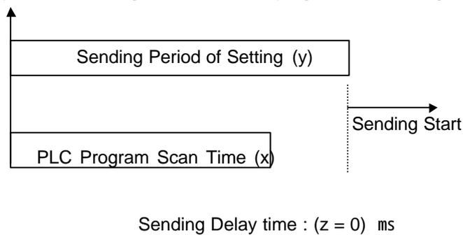
b. Delay time of sending data when PLC program scan shorter than sending period.
