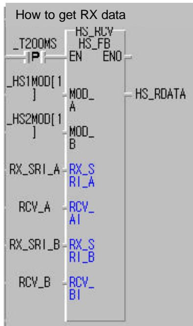
**\_T200MS:** must be identical to RX period of RX parameter.
