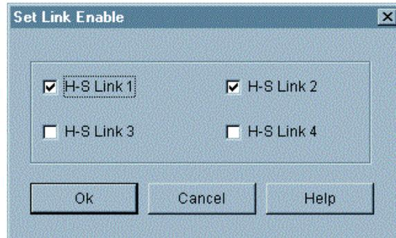
J) Confirm whether the communication for the set parameter is normally operating by selecting , On-line/Link parameter' and Monitor/HS\_LINK1 after positioning PLC mode as RUN.
