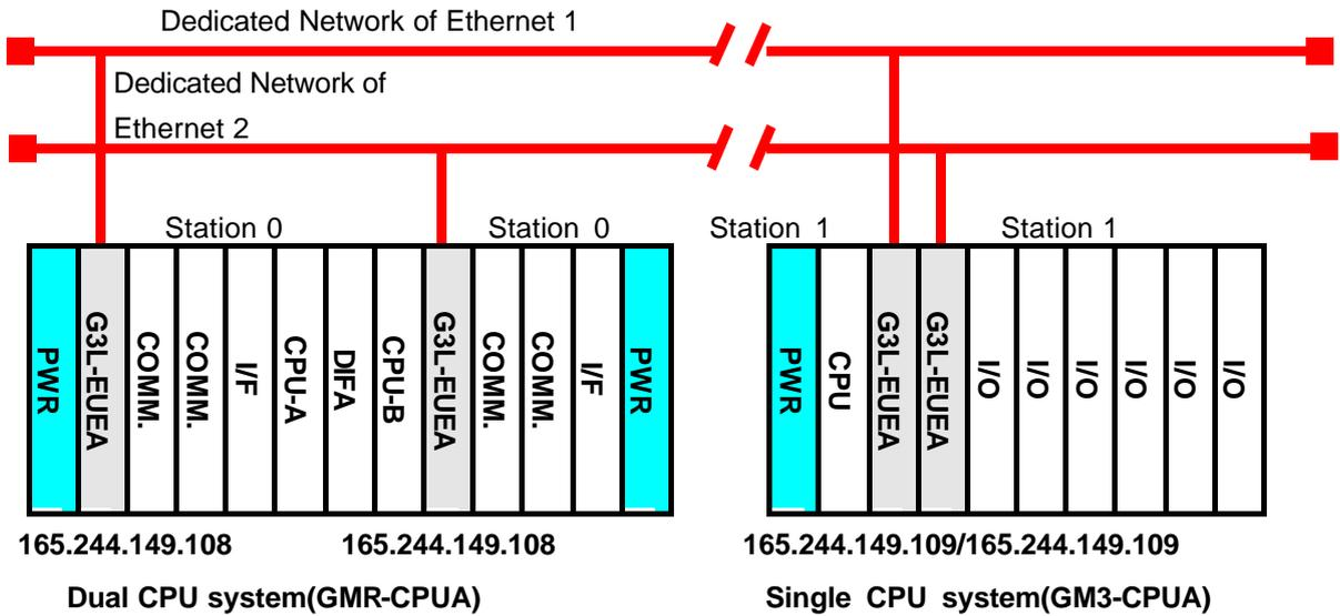
[Figure 7.3.3(A)] Redundant CPU and Network redundancy of GM3 PLC
