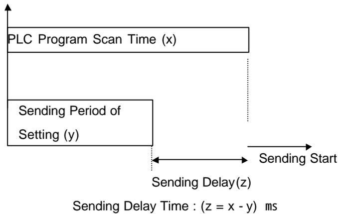
a. Delay time of sending data when PLC program scan is longer than sending period.
