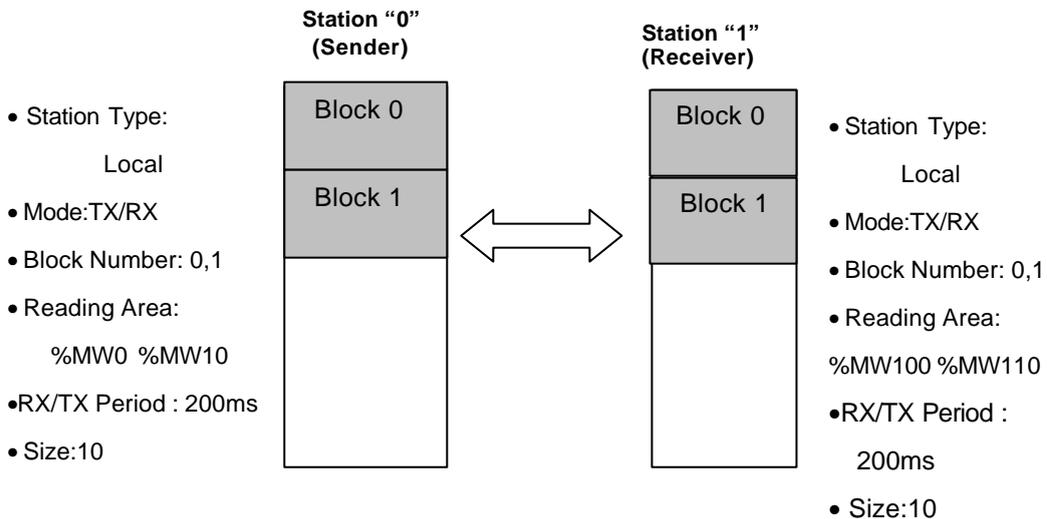
[Figure 7.2.1(A)] Block Diagram of Data Flow
