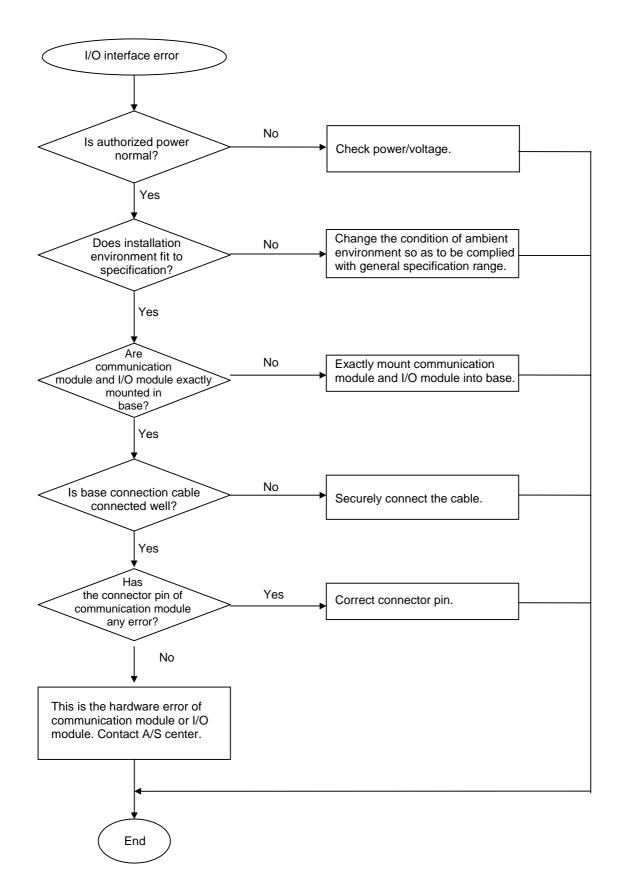
9.2.6 Error code E02-02 : Slave mounting and writing interface error during operation
