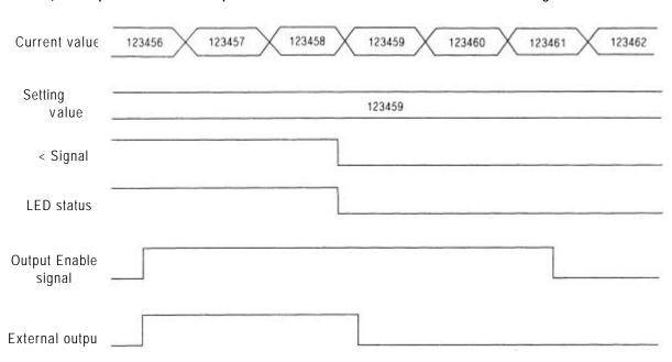
1) Example When the Comparison Mode Is Set to 'Current Value < Setting Value'
