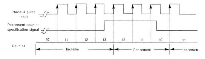
2) 1-phase Operation Mode (Increment /Decrement Count by Phase B Pulse Input)
