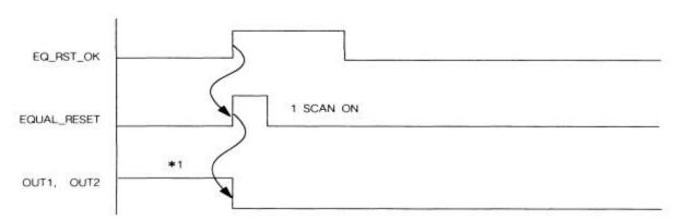
\*1. This occurs only when the comparison values 1 and 2 are set to "=", "  $\geq$  ", or "  $\leq$  " and the current count value (CNT) equal to the comparison value (CMPD)
