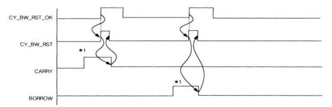
\*1. Carry, Borrow signal occurs when the Current count value changes from 16,777,215 to 0 from 0 to 16,777,215
