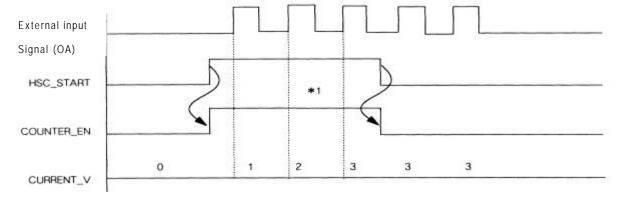
\*1. The current count value (CNT) is read only when the COUNTER\_EN is turned on.
