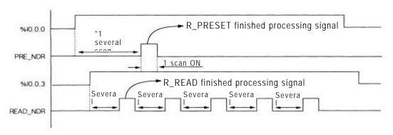
\*1. It is normal communication complete cycle, and it extents in proportion with quantity of communication data and the number of stations connected to the communication module.
