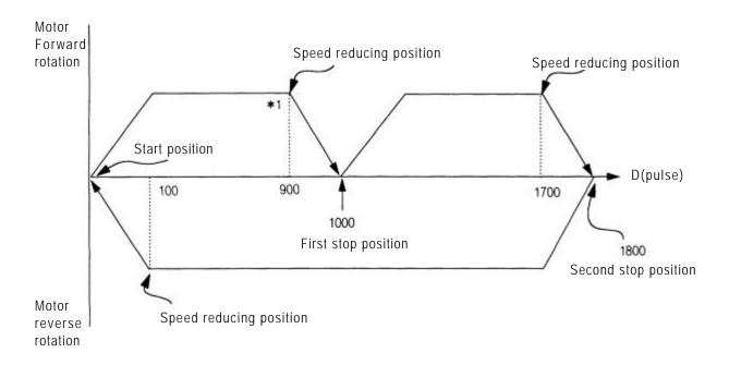
\*1. 100(Difference between stop position and speed reducing position) is an interval delayed by reducing timing of the inverter.
