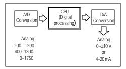
[Fig. 1.3] Processing in the PLC
