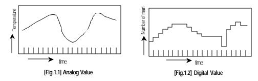
Continuous changeable quantity such as voltage, current, temperature, velocity, pressures and flux is called an analog quantity. For example, temperature changes continuously with time as shown in Fig. 1.1. The PLC can process that continuous changeable temperature by use of the thermocouple input module.
