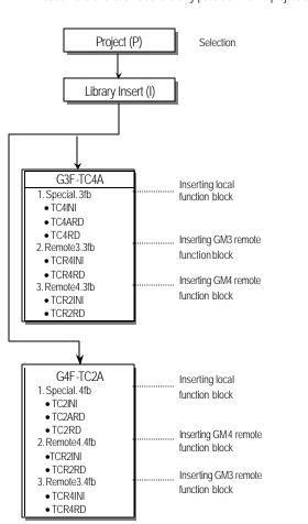
Function blocks can be registered with the following procedure while the GMWIN is running. Insertion of the function blocks is only possible when a project is open.
