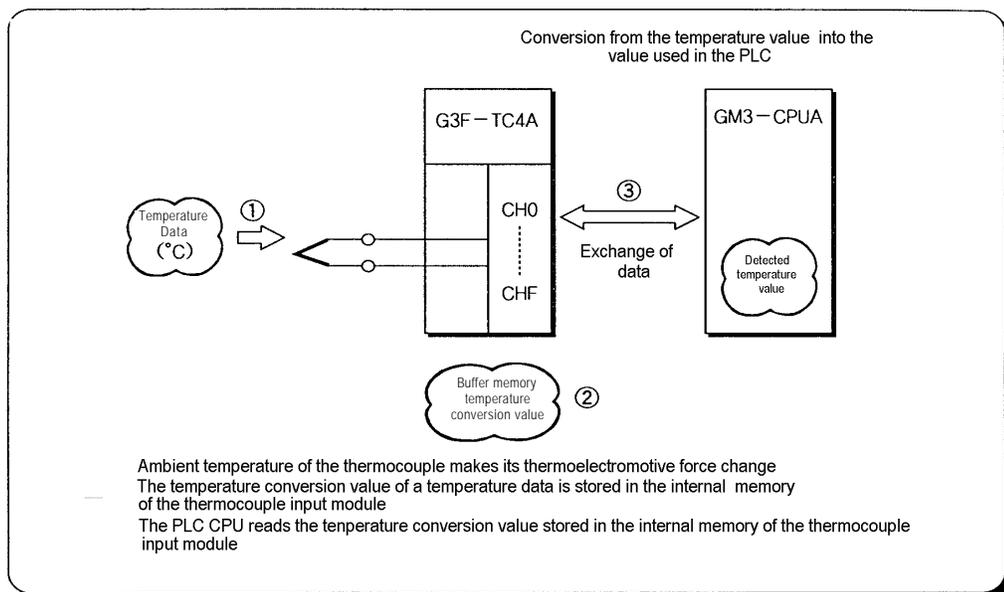
The thermocouple input module has following features.
