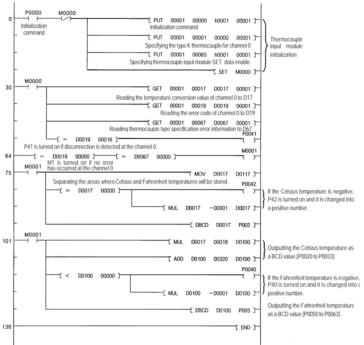
8.2.2 A Program for Magnitude Comparison of a Detected Temperature Value
