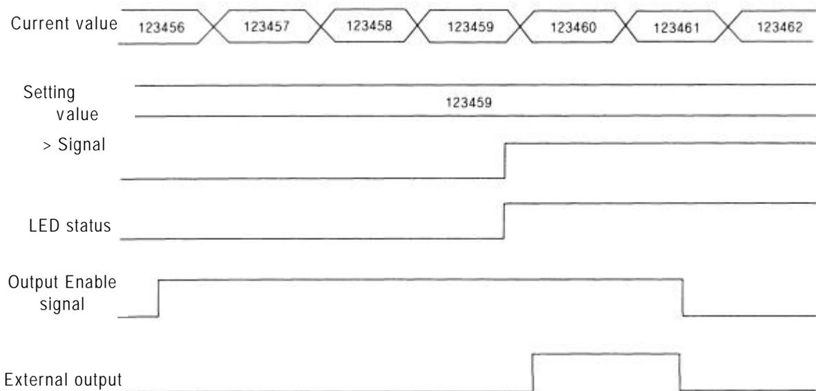
**3) Example When the Comparison Mode Is Set to 'Current Value = Setting Value'**
