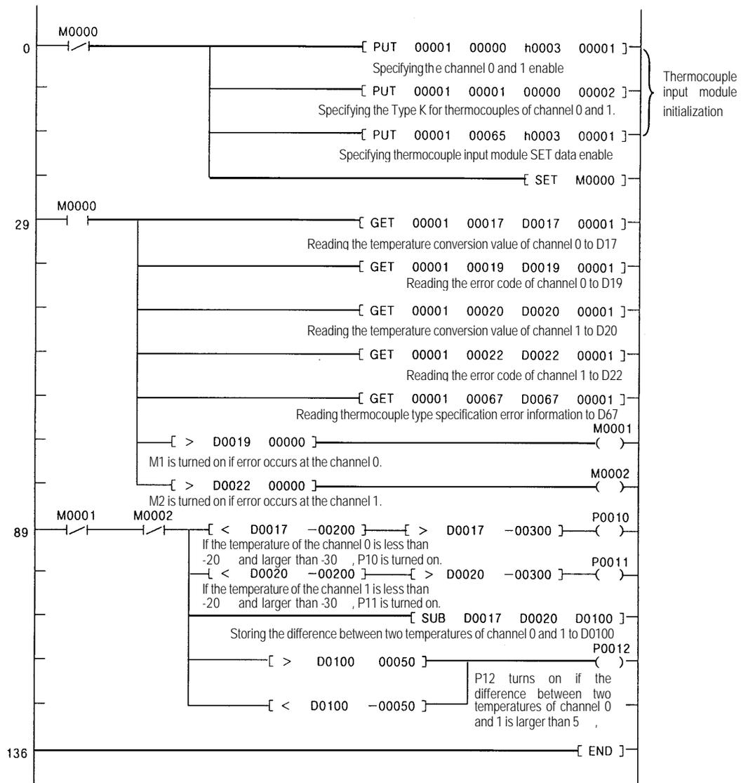
8.2.3 A Program Used When Mounting a Thermocouple Input Module on the Remote I/O Station
